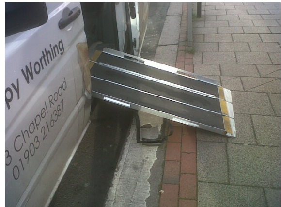
Photographs 2 & 3: Ramp being removed from the rear of the vehicle by the driver and placed in position for side loading access from the kerb:
