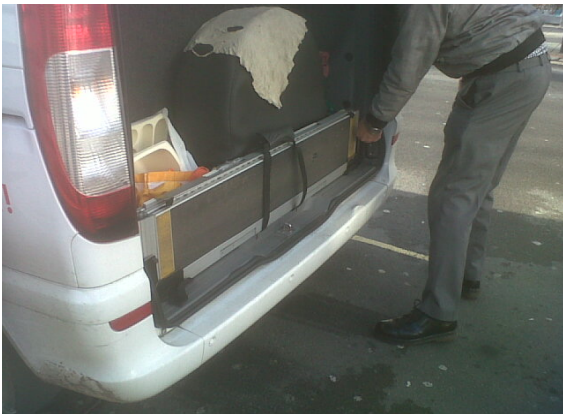
Photographs 2 & 3: Ramp being removed from the rear of the vehicle by the driver and placed in position for side loading access from the kerb:
